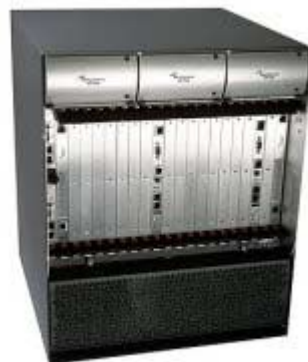
Figure 2: A Trunk Gateway (MetaSwitch MG3510)
